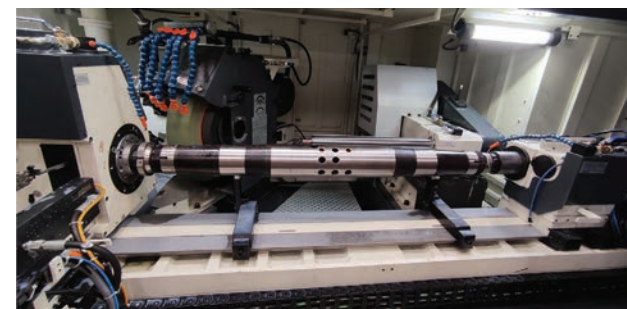
Figure 1: OD Grinding Set-Up
