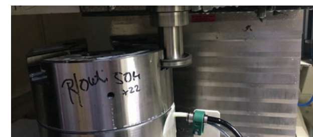
Figure 2: T-slot grinding with vertical grinding spindle
