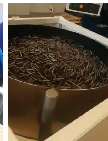
Figure 2: Rotary bowl for feeding components
