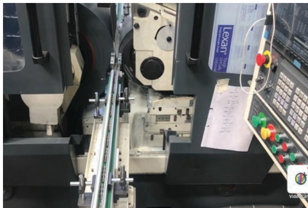
Figure 2: Component being fed by the conveyor for grinding.
