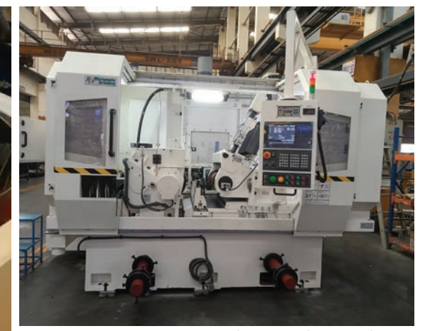
Figure 3: 6-Axis, CNC Centreless Grinding Machine, Twin Grip, CLG-6050TG
