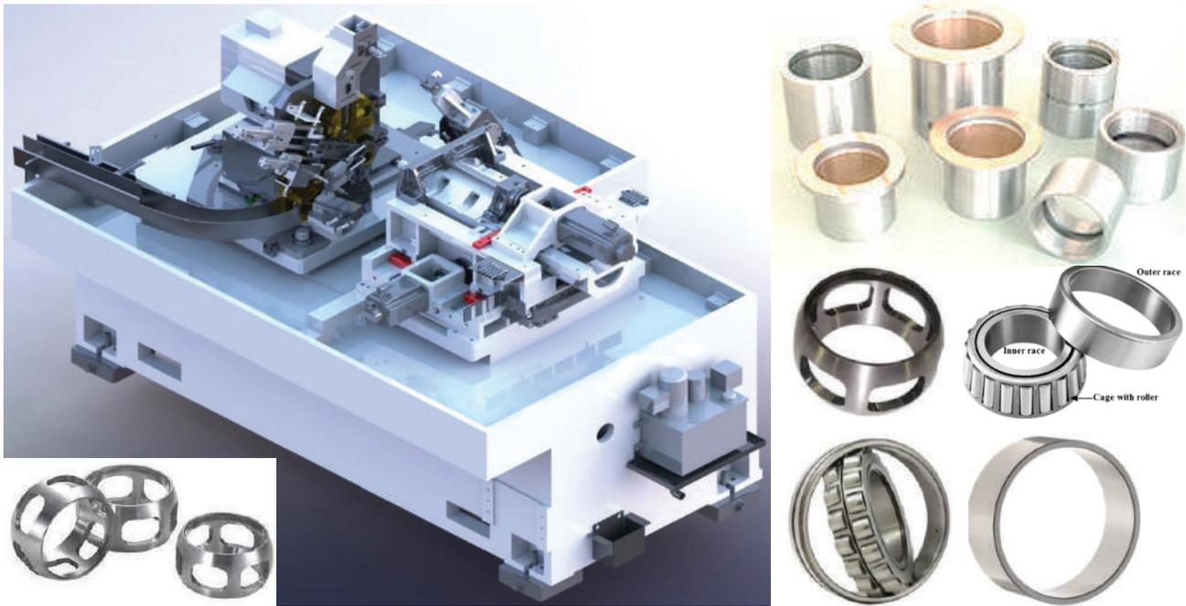
**B**EARINGS are extensively used in all the industries that require precise, vibration-free and noise-free motion as a key to performance. So higher the performance requirements, higher is the precision requirement of all the elements of a bearing. Some of the bearing elements like outer race and inner race are precision ground on a high-performance, high-speed automatic OD or ID grinding machines that are mostly imported from Europe, China or Japan.
