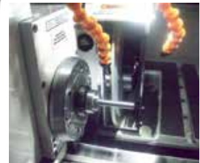
Carbide Blank Grinding on eco 200
