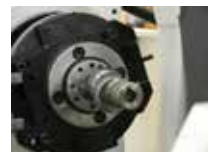
Compressor Eccentric Shaft Pin grinding using MGT's special fixture on GCE 350
