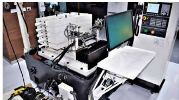
Hydrostatic Slide Testing Rig installed at AMTDC-IITM
