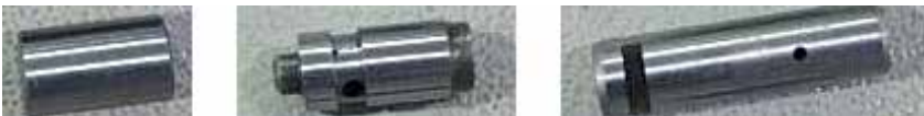
Plunger, Delivery Valve, Metering Valve (in that order), which basically are cylindrical rollers used in fuel pump assembly.
